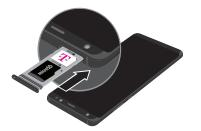
4. Slide the SIM card/Memory card tray back into the slot.
