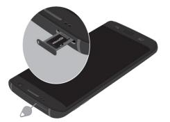
3. Slide the SIM card/Memory card tray back into the slot.
