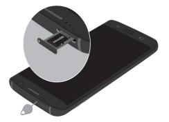
3. Slide the SIM card/Memory card tray back into the slot.
