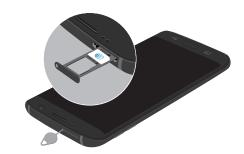
**Caution**: Be careful when using the removal tool to eject an internal card tray.
