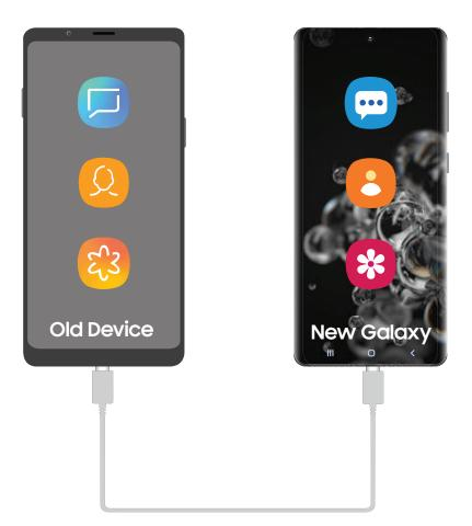
NOTE Transferring content with a USB cable may increase battery consumption. Make sure your battery is fully charged.
