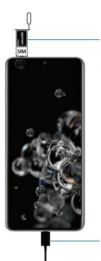
Install SIM/microSD card Place the SIM card and optional microSD card (sold separately) into the tray with the gold contacts facing down.
